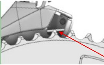
**Step 1: Height** - With chain in small ring adjust the height of front derailleur so that the outer plate of the derailleur cage clears the tallest tooth of the large chain ring by 1-2mm (or use the guide line). Use the inner limit screw to position the outer derailleur plate. Ensure cable anchor bolt is loosened.
