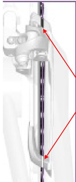
**Step 2: Turn the inner limit** (the one nearest the bike frame) screw while pedaling until the chain shifts up into the large chain ring. If necessary undo the outer limit screw a few turns.
