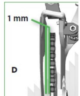
**Step 5: Anchor the front derailleur cable.** Make sure the the changer is in the large chain ring position before pulling cable tight and anchoring the cable with the anchor bolt.
