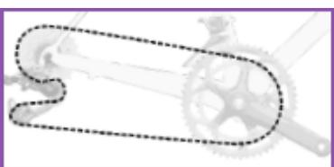
**Step 8: Install chain watcher** so that it is as close to the chain as possible when the chain is in the small chain ring up front and the large cog in the back without the chain watcher actually touching the chain. Slacken the fixing screw slightly and tweak the adjuster screw while applying inward pressure on the watcher then tighten fixing screw.
