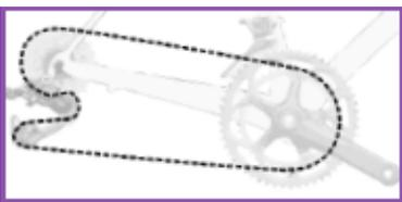
**Step 6: Set inner limit.** Use the shifter to release the cable tension by downshifting as you would for a shift into the small chain ring. Shift the rear derailleur into the largest cog. Back off the inner limit screw while pedaling to shift the chain down. Continue to back off the inner limit screw until chain noise disappears then turn screw another 45 degrees.
